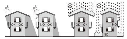
▶ Please make sure the inverter is installed at the right place. The inverter can't install close to trunk.
