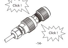
5. Finally, insert the AC connection plug into the AC connection receptacle on the inverter.
